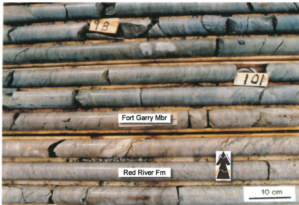
Photo 11: WL-92-51: Close-up of the contact between the Fort Garry Member (upper Red River Formation) and the lower Red River Formation (see Photo 10b).
