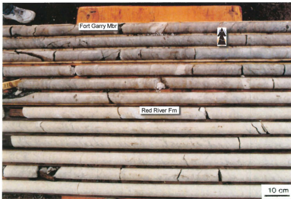
Photo 12a: WL-92-51: Contact between the Fort Garry Member and the lower Red River Formation. The lower Red River Formation becomes a lighter brown, dolomitic wackestone at its base (less argillaceous content).
