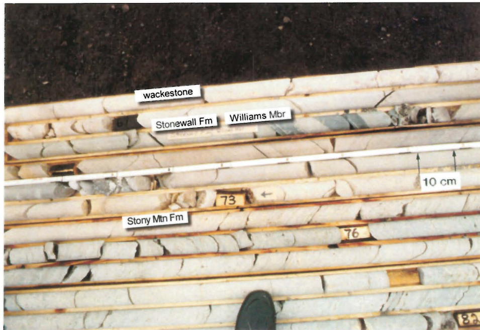
Photo 4a: WL-91-29: The contact between the Williams Member and the Stony Mountain Formation (arrow). The Stony Mountain Formation is a distinctly nodular to burrow mottled wackestone.
