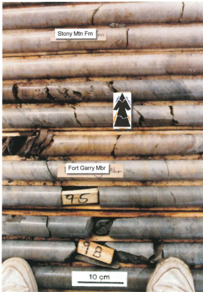
Photo 9: WL-92-51: Contact (at arrow) between the Stony Mountain Formation, a nodular wackestone, and the Fort Garry Member (upper Red River Formation), a massive to laminated mudstone.
