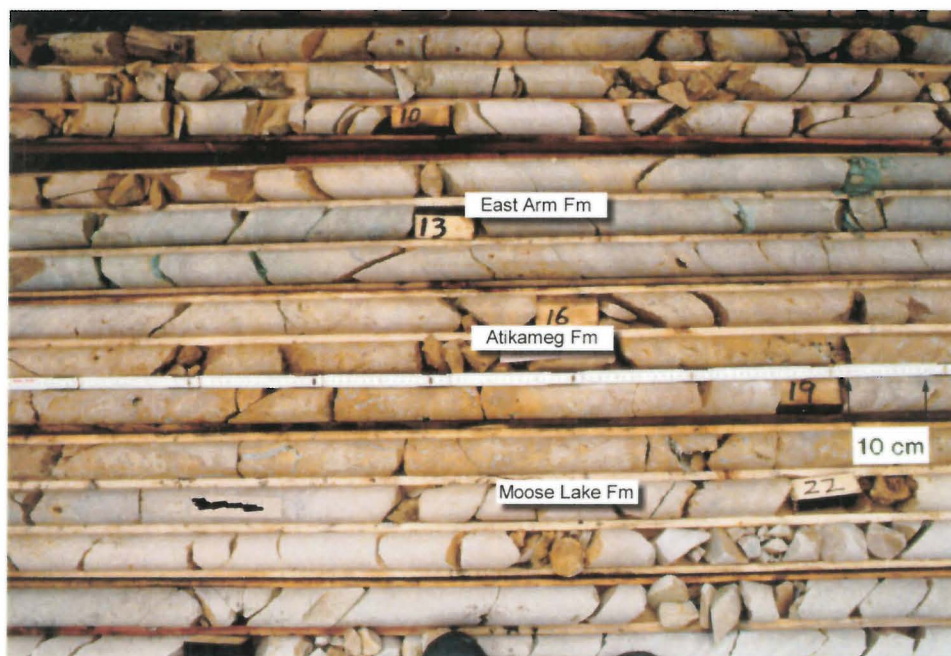
Photo 1b: WL-91-29: Contact between the Atikameg and Moose Lake formations. Note the very vuggy/porous texture of the Atikameg Formation and its buff orange colour. The contact to the Moose Lake Formation occurs at the base of a marker bed.
