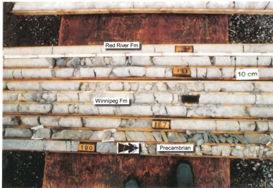
Photo 6a: WL-91-29: The Winnipeg Formation contact to the Precambrian. Intermixed lithologies of dolomitic sandstone, sandstone and siltstone (especially at the base). There is a sharp contact to weathered Precambrian at the base (just below the 190 m tag) (at arrow).
