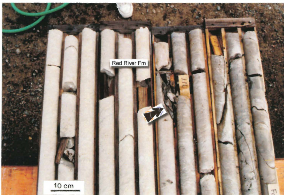
Photo 14b: WL-92-51: Clay infilled fracture (at arrow) and brittle fractures at 107 m (Red River Formation).
