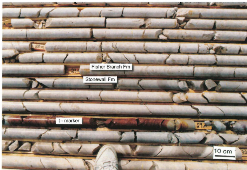
Photo 7b: WL-92-51: Contacts between the Fisher Branch and Stonewall formations, and the t-marker. There is a very sharp break between the Fisher Branch Formation and the Stonewall marker, and is well displayed in the photo. The t-marker, which occurs above the 29 m tag, is a distinctly red, laminated mudstone. This marker is not always red and may appear green to grey in colour (see Photo 2b).
