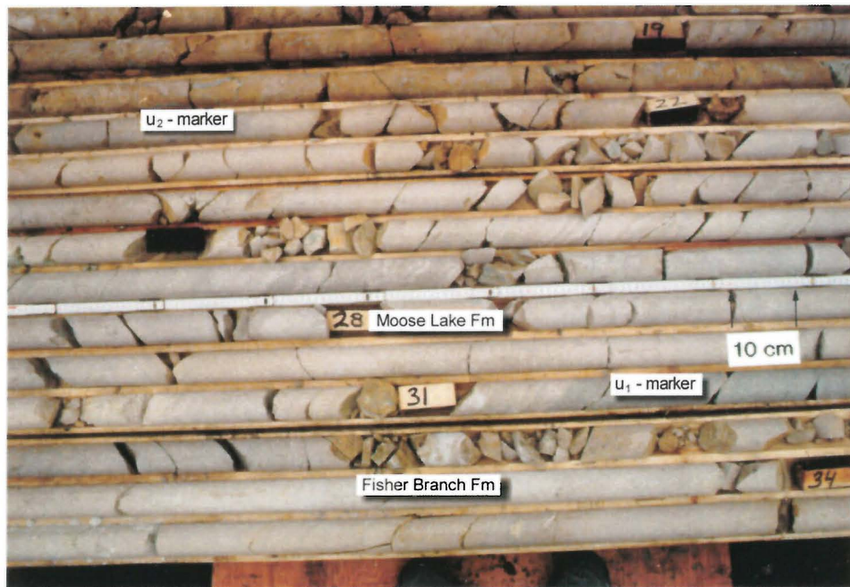
Photo 2a: WL-91-29: The Moose Lake, u_1 -marker, and Fisher Branch contacts. The Moose Lake Formation is a light brown to tan, massive dolomitic mudstone to grainstone. There is a distinct change to the u_1 -marker, which is a grey mudstone.
