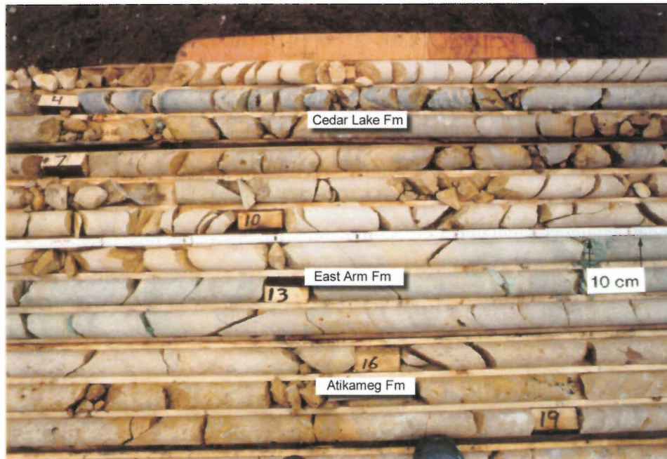
Photo 1a: WL-91-29: Contacts between the Cedar Lake, East Arm and Atikameg formations. The Cedar Lake Formation, present at the top of the hole, has a gradational contact to the East Arm Formation (this is a very uncertain pick). At approximately 13 m, the texture becomes a darker mudstone and probably represents the u_2 -marker (which was not identified when the photo was taken). A sharp change between the u_2 -marker and the Atikameg Formation (brown vuggy dolomite) occurs at 15.54 m.
